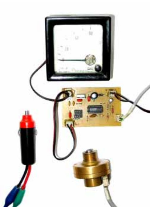
Fig. 5. The vehicle velocity transducer prepared to be mounted in the vehicle
