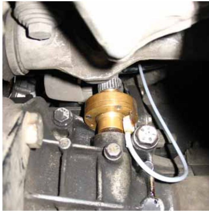
Fig. 6. The view of the transducer mechanical part mounted in the vehicle
